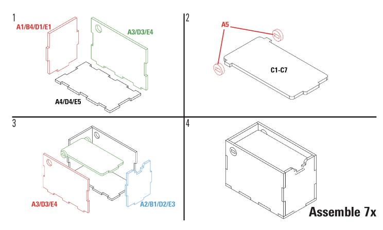
Required parts: **A1**x2,**A2**x2,**A3**x8,**A4**x4,**B1**,**B4**,**C1**-**C7**,**D1**,**D2**,**D3**x4,**D4**x2,**E1**x3,**E3**x3,**E4**x2,**E5**
