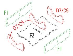
Required parts: **F2**, **F1**x2, **D7**x2, **C9**
